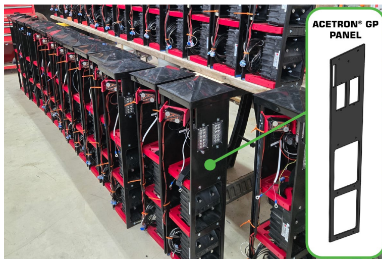
Figure 2 - RS-1A Cassette Acetron® GP Cassette Frame Panel
