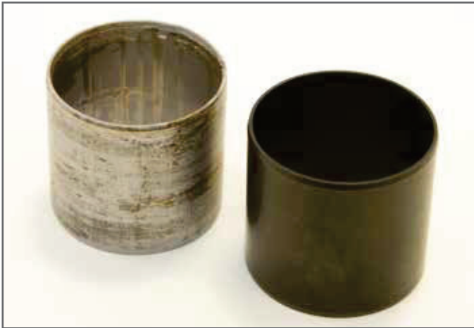
Duratron® CU60 PBI bushing next to the steel bearing it replaced due to shaft galling.
