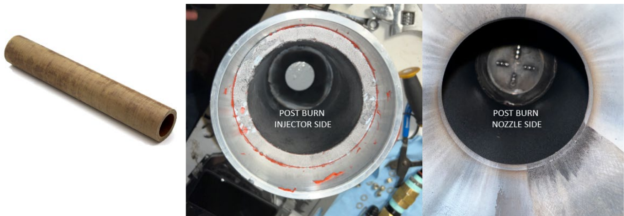
Figure 2 Phenolic CE Tube and Post Burn Photos of the Injector and Nozzle Sections of the Chamber show the charred ablative Phenolic Liner and Aluminum that protects as the SEB team test fired the rocket engine.
